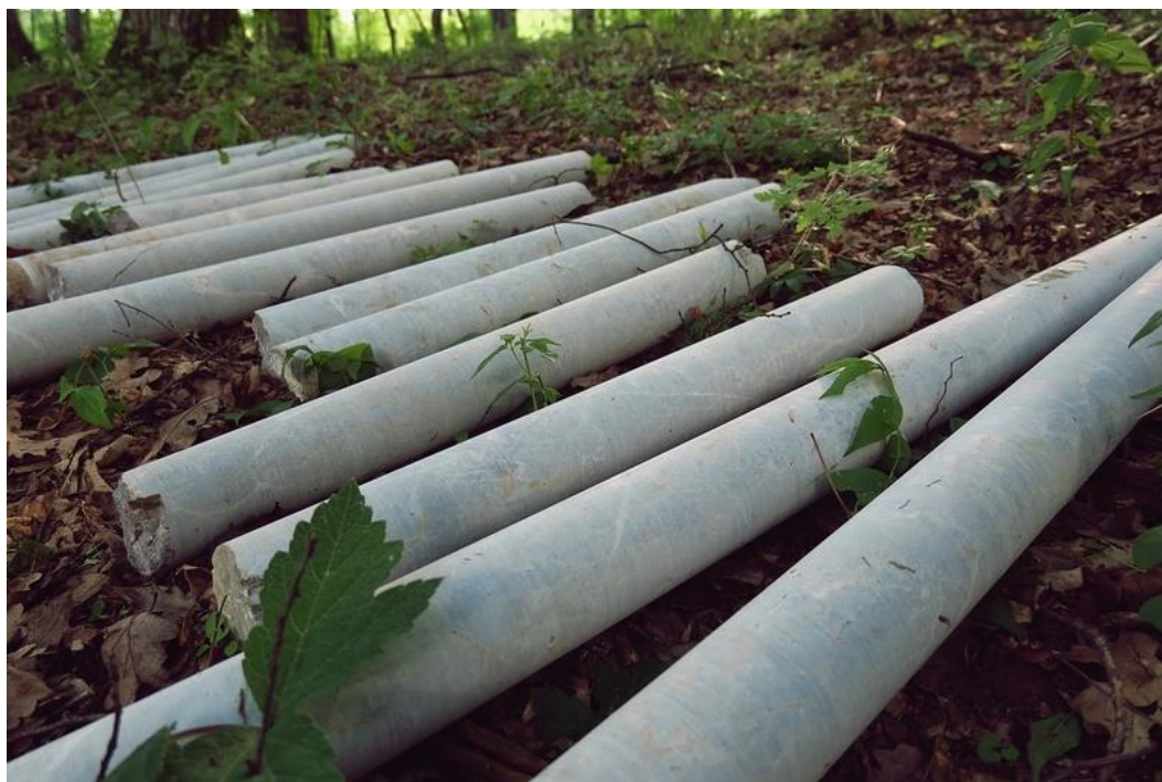
Obr. 3 Neporušené vrtné jadro z priestoru tunela Fig. 3 Intact drill core from the tunnel area
