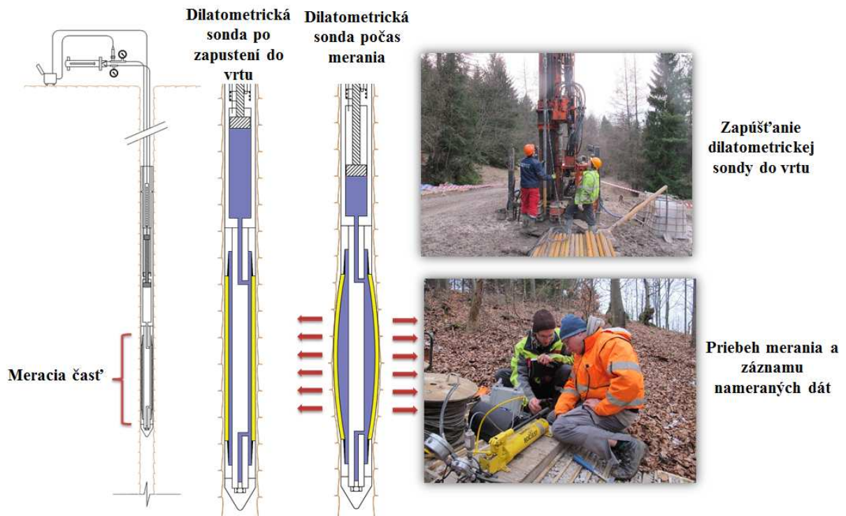
Obr. 2 Zapúšťanie dilatometrickej sondy do vrtu a meranie Fig. 2 Lowering of dilatometer probe into a borehole and measurement
