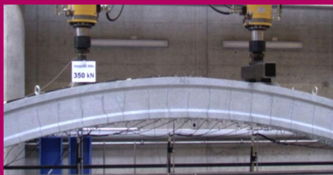
CRACK PROCESS SFRC.under a load 2 \times 350 kN.
