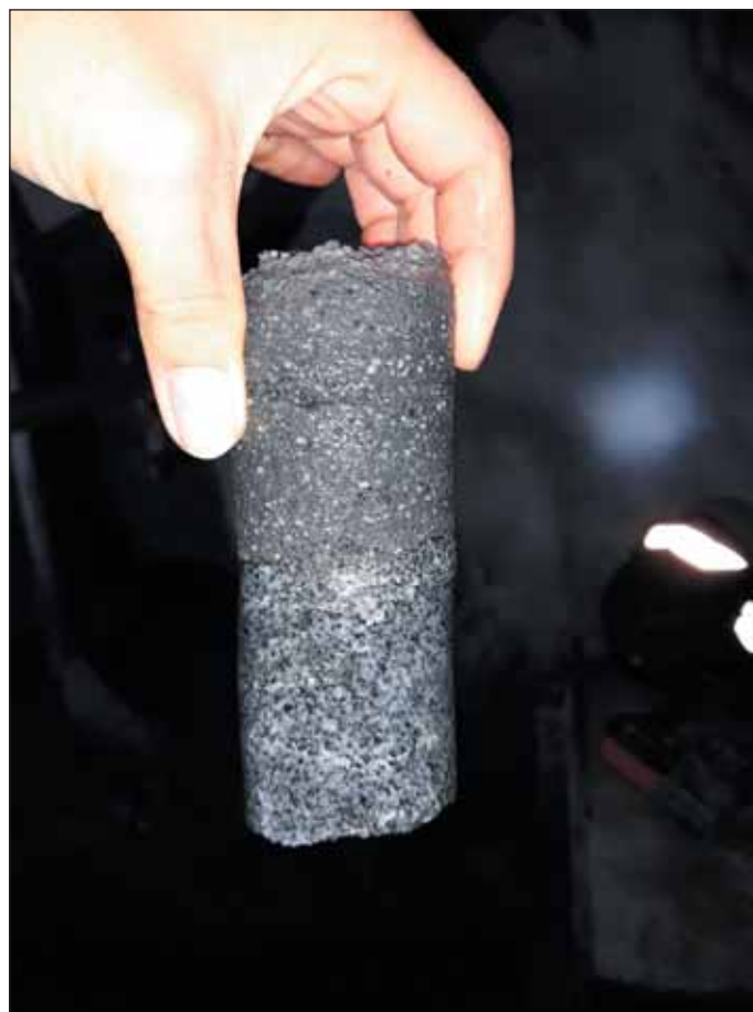
Obr. 8 Odvrtané jádro betonu s horninou Fig. 8 Drilled concrete core with the rock
