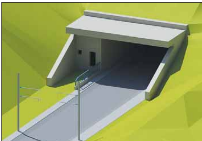
Obr. 6 Portál tunelu Sâtamyrikulverten – BIM model Fig. 6 Sâtamyrikulverten tunnel portal – the BIM model
