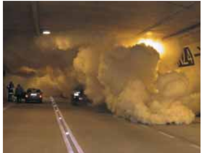
Obr. 5 Tvorba dymu v tuneli Fig. 5 Generation of smoke in the tunnel
